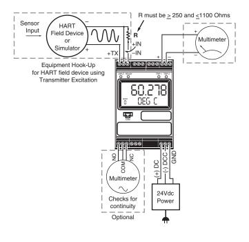
HART Communicator can be connected anywhere on the loop R must be  $\geq$  250 and  $\leq$ 1100 Ohms 24Vdc Power +၂-Sensor Input 4-20mA /// +IN -IN 000 000 000 000 HART Multivariable Field Instrument (Temperature Pressure, Level and Flow) Analog Output tied to Any Process Variable GND Event Recorder -(-) DCC 9 2 (+) DC NO (normally open) 24Vdc Power COMMON Source NC (normally closed)
