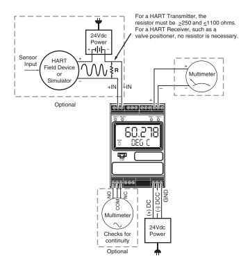
Figure 3. Bench Checking the HIM Using the Transmitter Excitation (+TX) Terminal to Power a Transmitter
